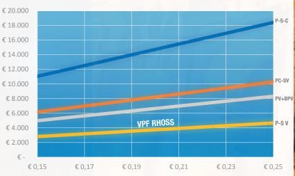
P-S-C Constant primary and secondary system PC - SV Constant primary and variable secondary
