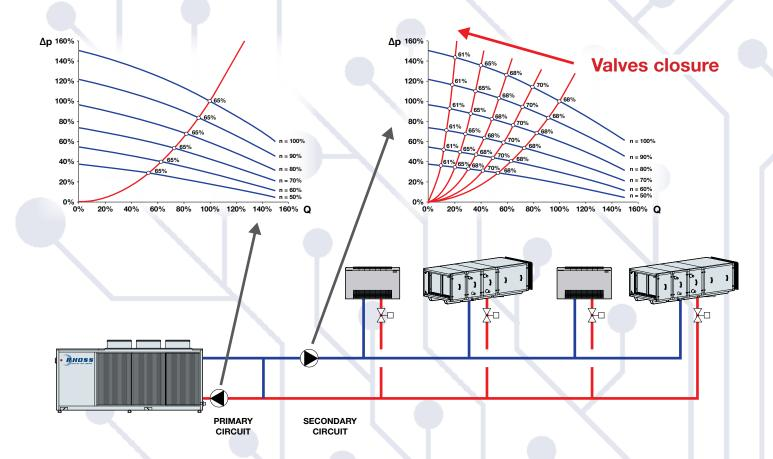
The concept is highlighted in the calculation formula below; it shows that the power absorbed by a pump varies mainly with the flow processed (Q) and the related head (Dp) and both dimensions depend on the pump rotation speed (n).
